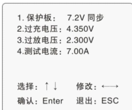
According to the above Settings, instrument will adopt 435 V above voltage test overcharge delay time, use 2.3 V under voltage tested put protection delay time, using 7A current test over-current delay time.
